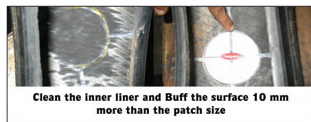
If repairable by Plug Patch mark the injury inside and outside. Check the size and angle of injury (angle should be less than 15°) and select the patch
