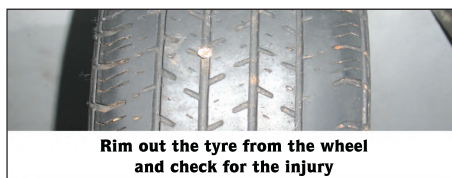
If repairable by Plug Patch mark the injury inside and outside. Check the size and angle of injury (angle should be less than 15°) and select the patch
