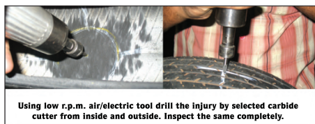
Rim out the tyre from the wheel and check for the injury
